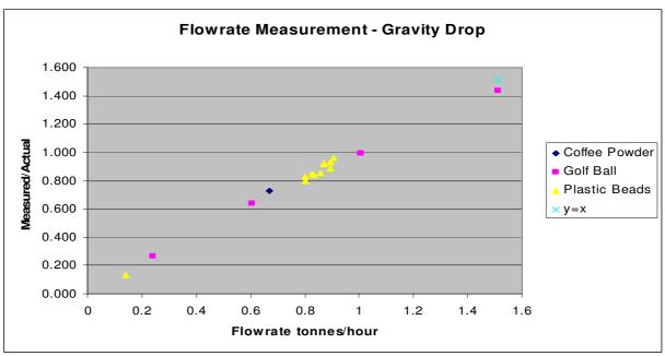
A summary of test results (above) for a range of flows indicates that Flowan calculates volumetric flow, converted here to mass flow rate, within typically a few percent of the true rate.
