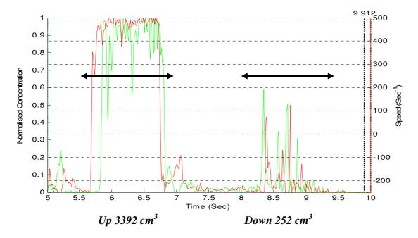
In addition to being able to integrate the total flowrate, the volume of individual structures within the flow may be calculated. For example in the slug flow shown above, the volume of the upgoing slug between about 5.5 and 7 seconds is 3392 cm<sup>3</sup>, equivalent to a 2 metre long plug of solids moving at about 200 cm/s over 1 second. The downward flow, although lasting just as long from about 8 to 9.5 seconds, only contains 252 cm<sup>3</sup>.
