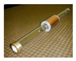
Data from the Tomoflow R100 system may be saved to file for off-line flow structure analysis using Tomoflow's Flowan multiphase flow analysis software. Example results are given here for several flow conditions in a 50mm diameter pipe. The sensor used is a twin-plane unit with 3cm long electrodes axially separated by 10cm driven guard electrodes. The sensor is shown in the photograph mounted on a 50mm perspex pipe ready to be mounted in the test rig.
