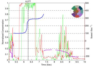
The velocity at each point in time within each zone is calculated by correlating the instantaneous concentration of one plane with the same zone in the other plane. result is plotted as a second graph with axes in cm/second on the right hand side of the graph. The blue line shows velocities this positive (in case upwards) and the mauve line shows downward velocities. It can be seen in this case that the slug front is moving at 100cm/s bur the tail is progressing at 300 cm/s.
