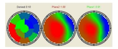
Flowan can calculate a number of average parameters for each zone, including average concentration and average flowrate. The example shows average concentration (left) over several 10s of seconds, compared with the instantaneous images (middle & right).
