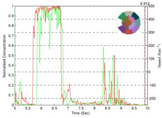
The first half of the graph shows upflow - an upward-going slug with concentration going from near 0 to near 1 in a short space of time at plane 1 (red line) slightly before arrival at plane 2 (green line). It can be seen that the rear of the slug is travelling faster than the front. On the second half of the graph the green line shows concentration events at plane 2 (upper) preceding their arrival at plane 1 (lower plane - red line).
