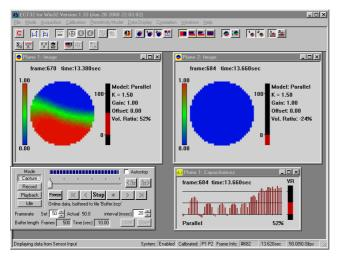
**ECT32-3.** ECT32-3 is a comprehensive on-line software suite for controlling and processing data from Tomoflow and PTL ECT systems. The software runs on the Windows operating systems. The images can be shown on the screen in real-time, then recorded and played back at user-defined speeds. Data files can be used for flow analysis using *Flowan\**.
