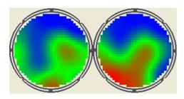
Images of flows are shown as circular maps with a grid of 32x32 pixels using a colour scale from blue (pixel empty) to red (pixel full). The example alongside shows the arrival of a slug front in a horizontal flow of plastic pellets in air. In this case the leading plane is on the right. Flowan automatically establishes the direction of flow.
