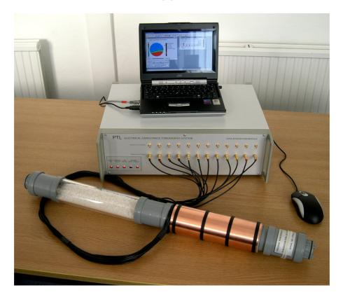
Following the development of our new **TFLR5000** very high-speed ECT system, we have a limited number of our previous generation ECT systems available for sale. These are complete single-plane 12-channel ECT systems, supplied with a Windows 7 or XP laptop PC, full set of control and analysis software and a basic 12-electrode ECT sensor. Custom capacitance sensors can be supplied if required at additional cost.
