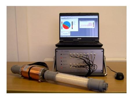
The **TFLR5000** is a high-speed Tomographic imaging system and Flow Anayser. It can be used for imaging, analysing and measuring the distribution and flows of mixtures of 2 non-conducting materials and is based on the use of Electrical Capacitance Tomography (ECT). Data can be captured at rates up to 5000 image frames per second.
