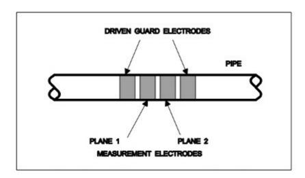
Figure 1. Principle of flow measurement using ECT
