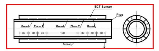
Figure 2. Cross-sections of 8-electrode twin-plane ECT sensor
