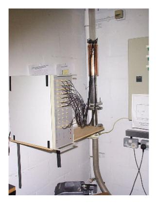
Figure 3. ECT sensor in vertical section of flow rig
