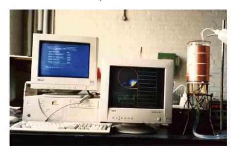
An early ECT system imaging water droplets in kerosene.
